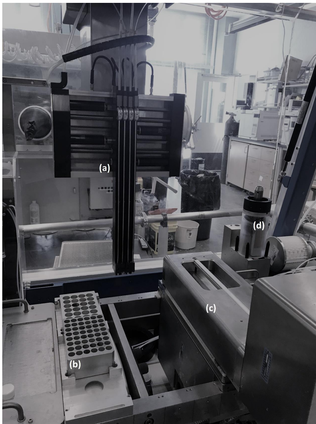
Figure S3. Close-up image of Chemspeed SWING-XL MTP Block. a 4-needle head solvent dispensing system b MTP block vial racks c MTP block reactor d Gripper tool
